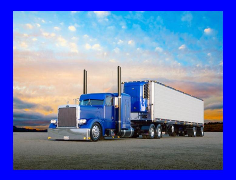
Since they have no front wheels and are depended upon connecting to a truck. Trailers are automatically locked when standing alone. The pressure from the truck air pump releases the trailer brakes when it is connected.
